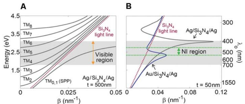
**Fig. 1.** Implementation of positive- and negative-index MIM waveguides. (A) Calculated dispersion curves for an Ag-Si<sub>3</sub>N<sub>4</sub>-Ag waveguide with a dielectric core thickness  $t = 500$  nm. (B) Calculated dispersion curves for Ag-Si<sub>3</sub>N<sub>4</sub>-Ag and Au-Si<sub>3</sub>N<sub>4</sub>-Ag waveguides with  $t = 50$  nm.
